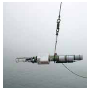
Deployment of a Pro-Ice (equipped with BGC sensors) in Baffin Bay (BB2 site, July 2017, from the Amundsen, AN1702 mission). © Claudie Marec
