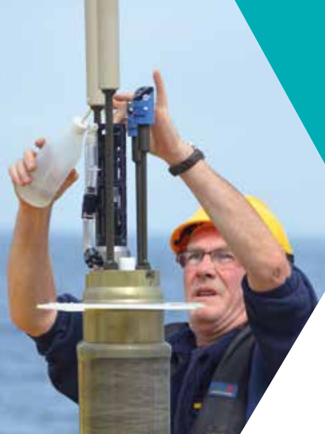
Deployment of a Deep-Arvor float. © Kevin Balem/LOPS
