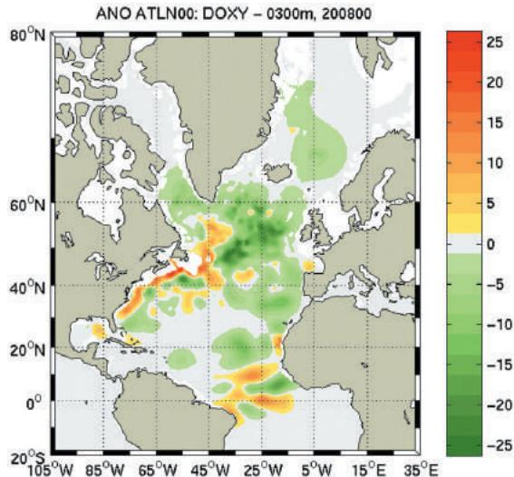
**21** DISSOLVED OXYGEN CONCENTRATION ANOMALY AT 300 M DEPTH COMPARED TO THE WOA09. ALL ARGO OXYGEN DATA AVAILABLE AT CORIOLIS GDAC WERE INTERPOLATED WITH ISAS TOOL.
