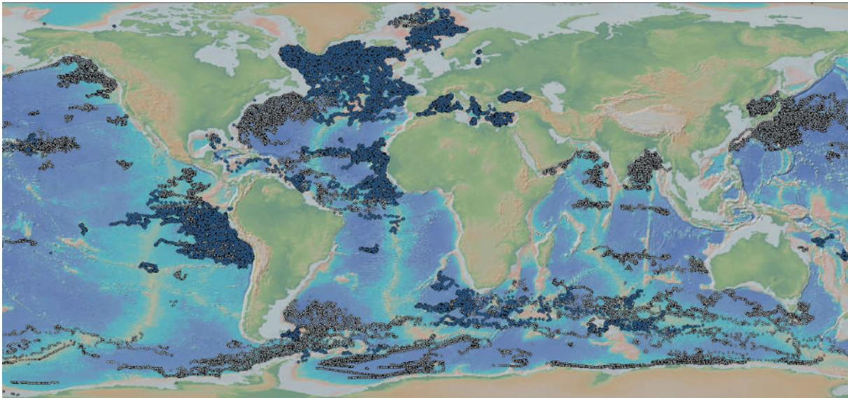
**22** MAP OF THE 294 BIO-ARGO FLOATS DEPLOYED BY E-AIMS AND OTHER EUROPEAN PROJECTS (BLUE DOTS). THE OTHER BIO-ARGO FLOATS (USA, AUSTRALIA, JAPAN, CANADA, INDIA) ARE SHOWN AS GREY DOTS. BIO-ARGO FLOATS MEASURE PARAMETERS SUCH AS OXYGEN, CHLOROPHYLL, NITRATE, PH, BACK-SCATTERING, RADIANCE, IRRADIANCE AND PAR.
