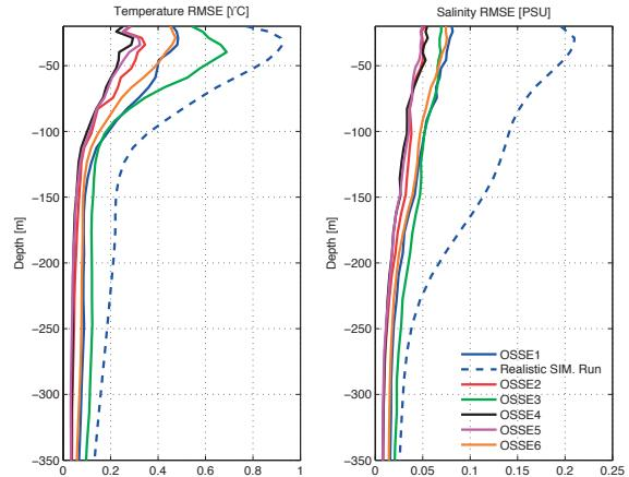
**15** RMSE OF THE ARGO MISFIT DURING THE 2012 FOR ALL THE MEDITERRANEAN SEA. BLUE LINE OSSE1 (5 DAYS DRIFT, PD 350M), RED LINE OSSE2 (5 DAYS DRIFT, PD 700M), GREEN LINE OSSE3 (5 DAYS DRIFT, PD 150M), BLACK LINE OSSE4 (3 DAYS DRIFT, PD 350 M) MAGENTA LINE OSSE5 (3 DAYS DRIFT, PD 700M) AND ORANGE LINE OSSE6 (5 DAYS DRIFT, PD 350 M, PERFECT VERTICAL SAMPLING).
